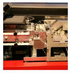
■ The Kern 3200 falsh offers the option of separately diverting both documents and empty envelopes during the inserting process. With these two options and the standard document monitoring system, the machine is able to divert faulty documents or envelopes preventively.
